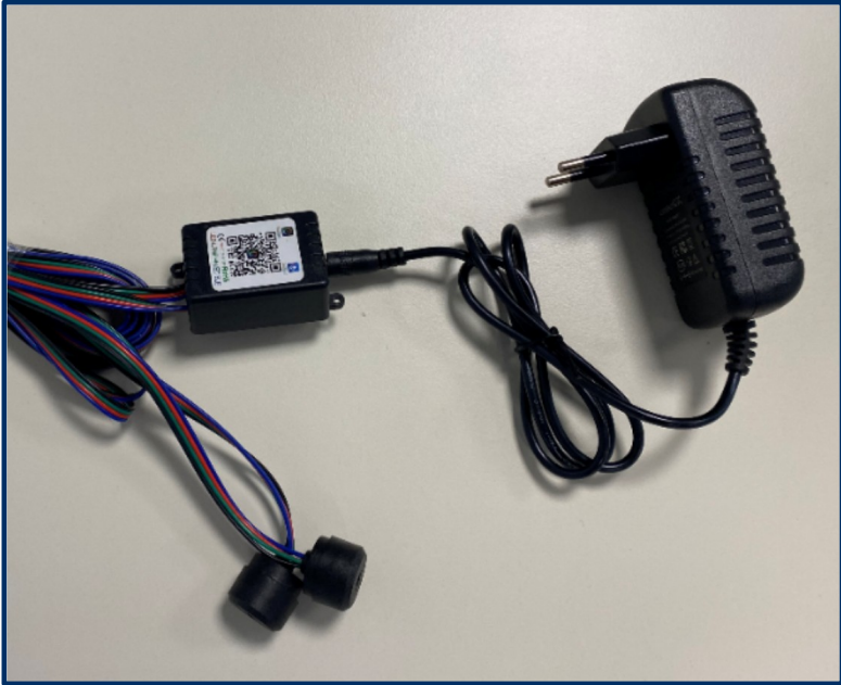
1: two LED-boxes on one controller for lenght up to 2 meters
