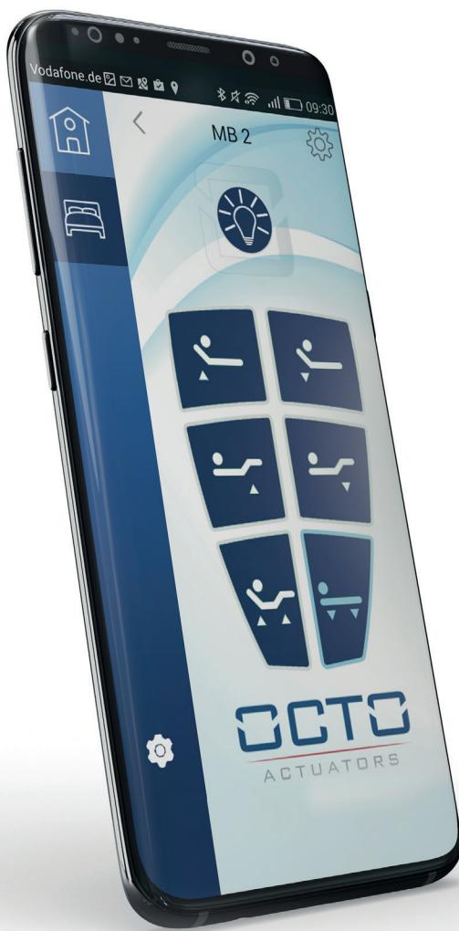
Operation via Bluetooth with a smartphone app. Night light function for smartphone app and classic radio control, also retrofittable
